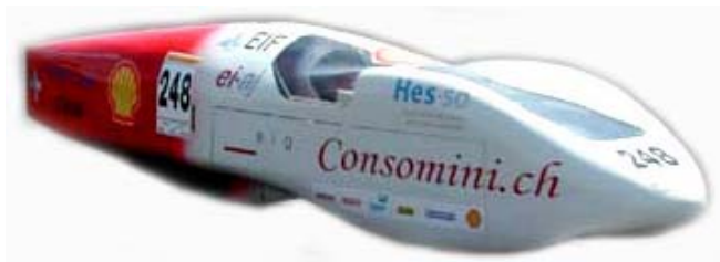
Fig. 1 : Consomini : A very high efficiency vehicle able to cover 1230 km with only one liter of traditional fossile fuel.
