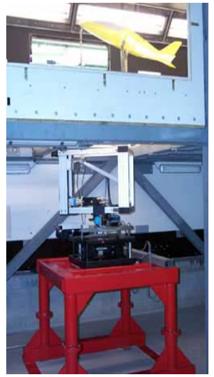
Fig. 16 : Examples of balances used to measure forces and moments until 6 components (3 forces and 3 moments simultaneously)
