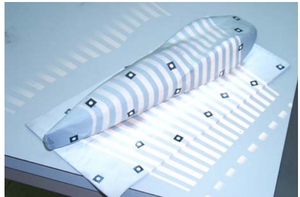
Fig. 4 : 3D scanning of the 1/8 scale model
