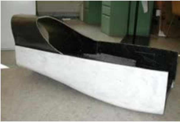
Fig. 3 : Body and frame are only one
