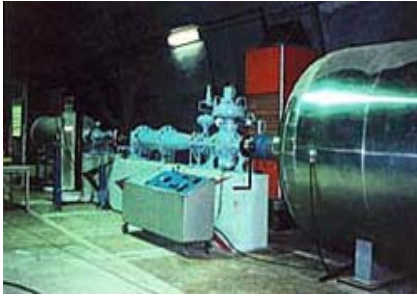
Fig. 14 : Supersonic wind tunnel (Mach 2.4)
