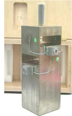
Fig. 16 : Examples of balances used to measure forces and moments until 6 components (3 forces and 3 moments simultaneously)
