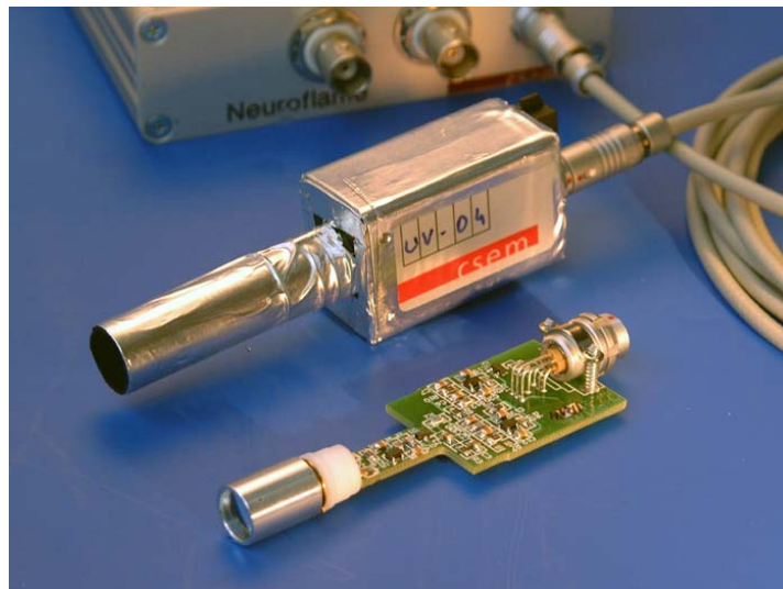
Figure 2 – Photograph of sensor and electronics
