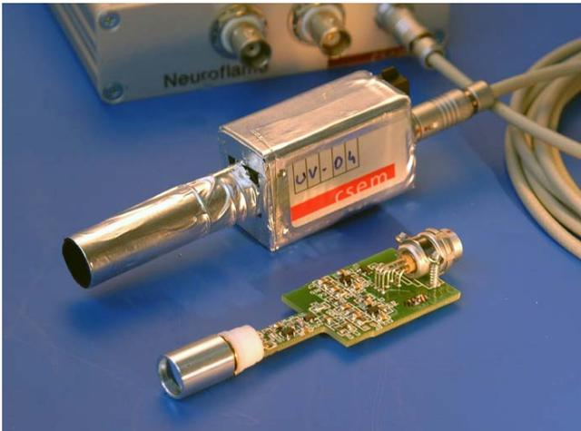
Figure 3 – Photograph of the flame signature sensor (by courtesy of CSEM)
