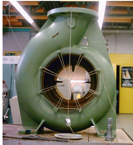
Figure 12b): Volute geometry measurements
