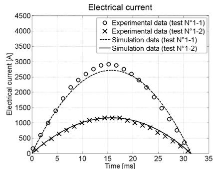
Figure 3: Measured (circle and cross marks) and calculated (dashed and solid lines) time dependence of electrical current, for fixed arc test 1-1 and 1-2
