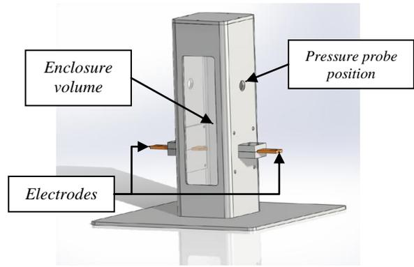
Figure 1: Geometry 1 (fixed arc), internal volume of 90x90x300 mm<sup>3</sup>
