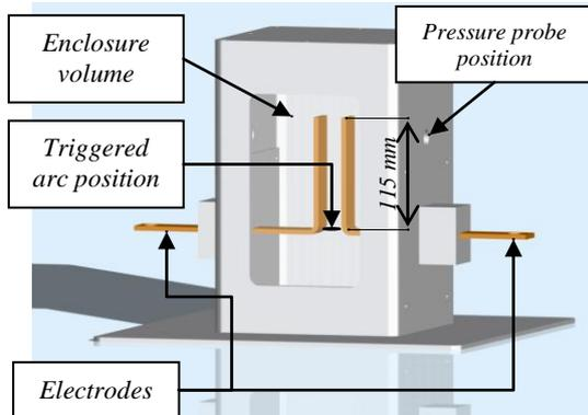
Figure 7: Geometry 3 (moving arc), internal volume of 180x180x300 mm<sup>3</sup>
