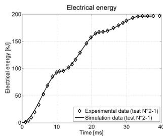
Figure 5: Measured (diamond marks) and calculated (dashed line) time dependence of electrical energy inserted inside the volume, for fixed arc test 2-1
