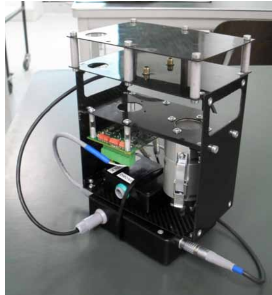
Figure 2. The metallic oxide NO 2 payload with 16 bits digitalizer and 2.4 GHz data link to ground station.
