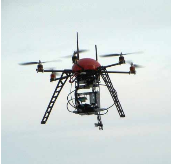
Figure 1. The hepia UAV equipped with the metallic oxide NO 2 payload.
