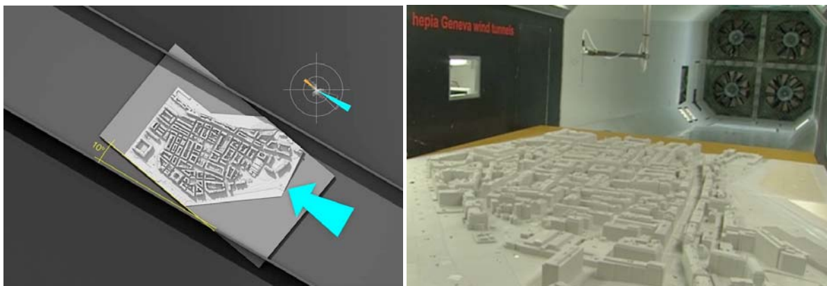
Figure 9. The 3D model in place inside the wind tunnel for SF6, wind speed fields, etc. measurements. On the top the SF6 gas inlet head connected to a 3 axes translator.
