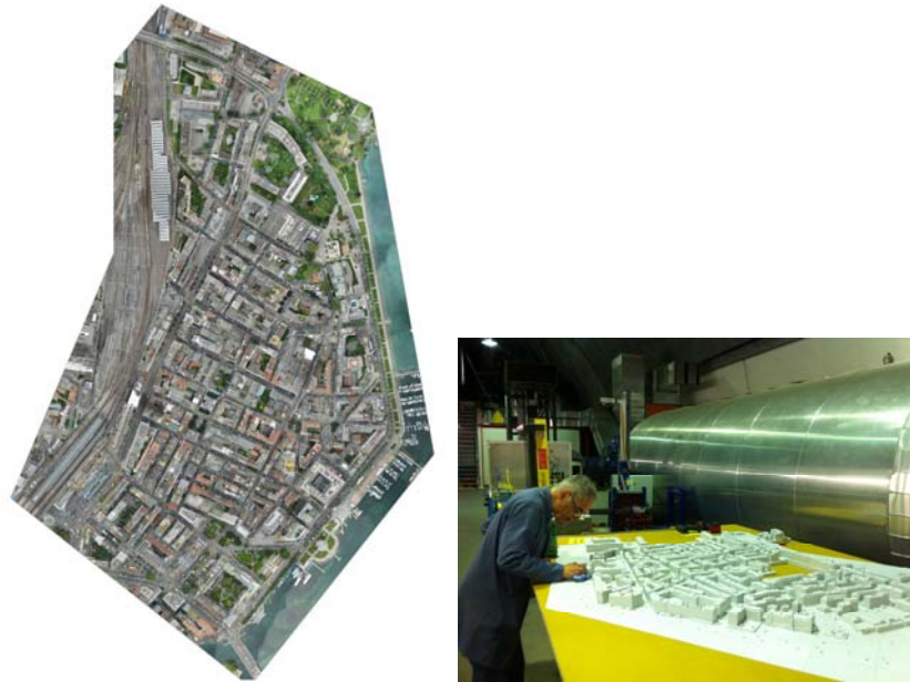
Figure 3. UAV image of the chosen region of interest (left) and the model during assembly (right).
