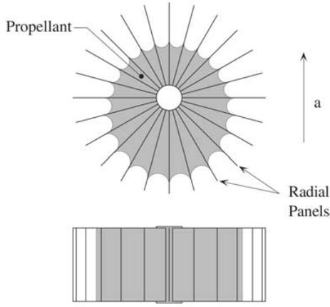
Figure 1. A “sponge” undergoing an acceleration. [1]
